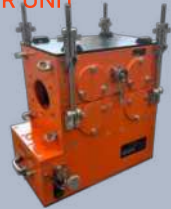
Remote device for actuating INTROS along inclined ropes
