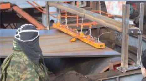
INSPECTION OF CONVEYOR BELTS
